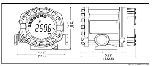
Die-cast aluminum housing for general purpose or, as option, stainless steel housing (316L) \* Dimensions without display = 4.41" (112 mm)
