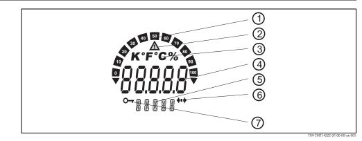
LC display of the field transmitter (illuminated, pluggable in 90°-stages)
